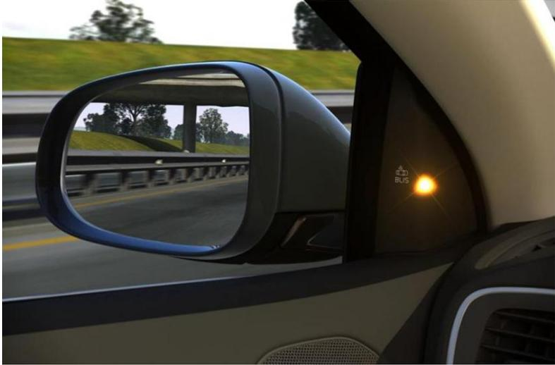
Figure 1.4: Volvo side-view mirror warning light indicating the presence of another car on the changing lane.
